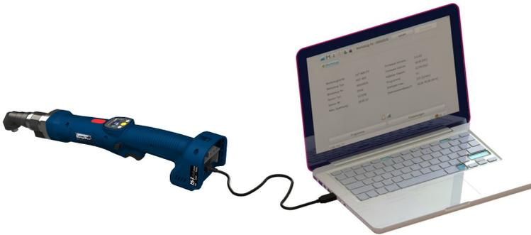
Start the HST-Tool-Manager, log in and read out the current tool by clicking on “read”. Now you can edit the settings as described in the following steps. So that the tool parametrization is not lost we recommend saving this separating under another name.
