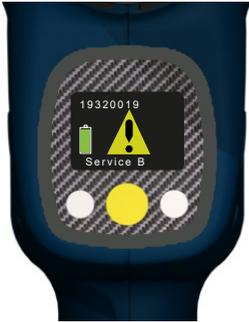
The service counters can be parametrised with the HST-Tool-Manager under the „Service“ user. The respective value entered will be multiplied by 1,000, i.e. when entering 10 the service notification will appear on the display after 10,000 sets. If you enter 0 the function is deactivated.
